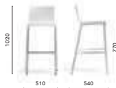
1116 Barstool, technopolymer shell, steel tube frame
