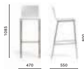
4415/KUTP Barstool, technopolymer shell, stainless steel central base
